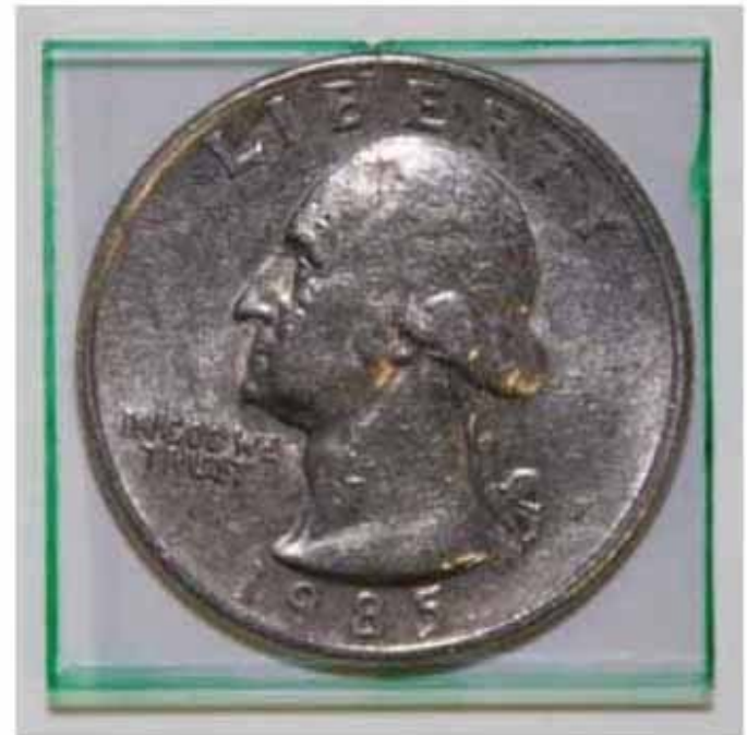
Photo of a 70-device array of fully transparent inorganic-organic hybrid thin film transistors on a 1"x1" glass substrate. The edges of the glass substrate are marked in green for clarity.
